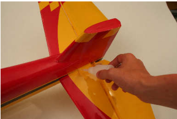
Picture 51: Elevator / glue
