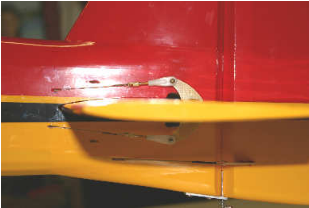
Picture 47: Elevator linking / Detail 2
