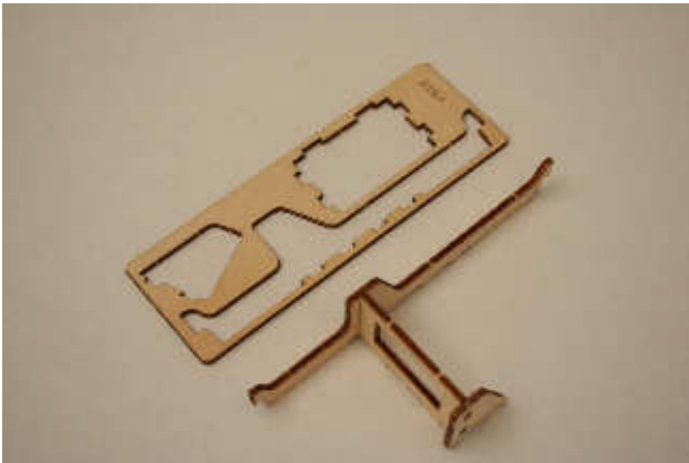
Picture 40: Elevator servoframe
