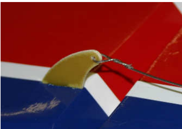
Picture 30: Rudder / Wire / secured loop
