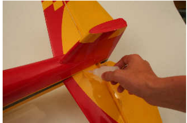
Picture 38: Elevator / glue
