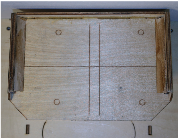
Picture 27: Firewall / markings
