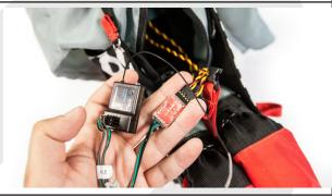
Place the receiver, the paramixer and the receiver battery inside the pilot's torso into the special location for that purpose.
