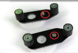
Mount the last silent block( this one hasn't an integrated threaded rod), with 1 CHC M3x8 screw. Do the same operations on the second horn.
