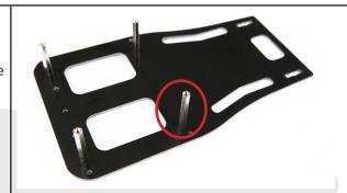
As shown on the picture on the right, affix 4 CHC M3x8 screws with 4 M3 nuts on the same plate. thos screws will have the function of holding the servomotors.
