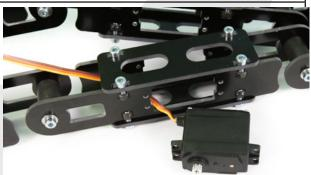
Lock the servomotor with 2 CHC M3x8 and M3 nuts.
