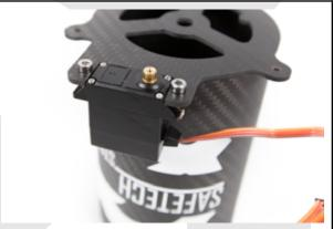
Use pliers to fold the ejection pin to an angle of 5°.
