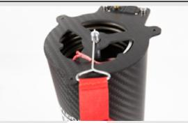
Arrange the horn on the servomotor. Push it up on the highest position. Then place the horn in the position shown on the picture.
