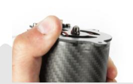
Lock the arming rod with the "Remove Before Flight" pin.
