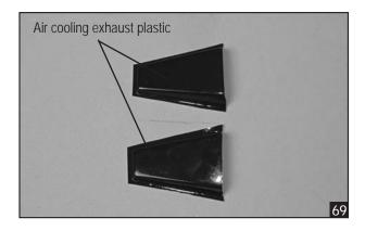
9. Cut the hole on the fuselage for installing the air cooling exhaust plastic.
