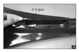
3. Install the steering nose servo into the servo tray in the fuselase.
