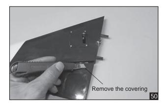
6. Install and glue the rudder control horn.
