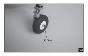
6. Secure the strut suspension to the retract.
