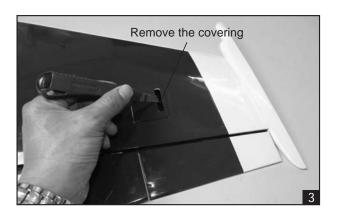
Place the servo into the servo tray. Center the servo within the tray and drill 1,6mm pilot holes through the block of wood for each of the four mounting screws provided with the servo.
