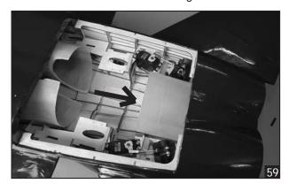
3. Trim 1 hole from the air outlet for the wires of EDF.
