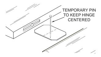
Apply six drops of thin CA to the top and bottom of each hinge. Do not use CA accelerator. After the CA has fully hardened, test the hinges by pulling on the aileron.
