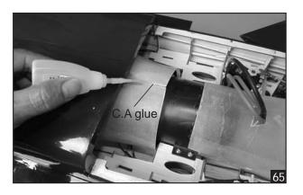
6. Glue the wooden belt for EDF (Included with the kit) using C.A glue.
