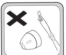
**NEVER** use damaged or deformed propellers or spinners.
