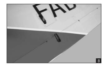
3. Repeat step # 1 - # 2 to install the second control horn on the aileron.
