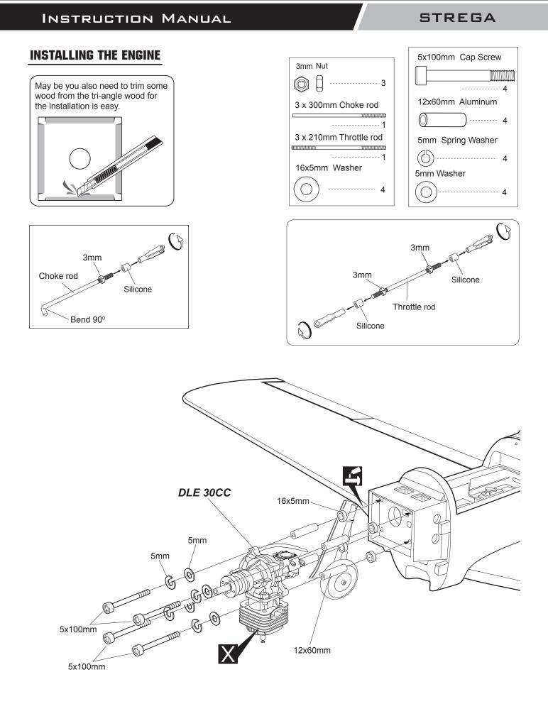
Apply threadlocker (screw cement).
