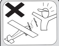
**ALWAYS** adjust the engine from behind the propeller, and do not allow any part of your body to be in line with the propeller.
