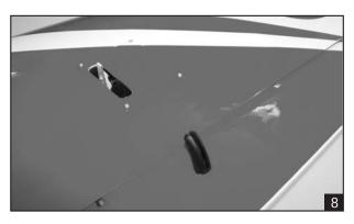
3. Repeat step # 1 - # 2 to install the control horn on the opposite aileron.
