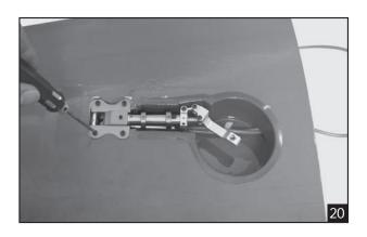
7. Pull out the air tube through the wing section.
