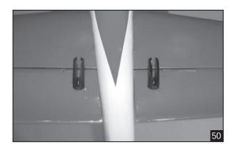
7. Attach clevis to the hole in the control horn.
