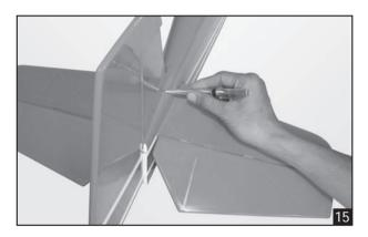
3. Now, remove the vertical stabilizer and using a modeling knife, carefully cut just inside the marked lines and remove the film on both sides of the vertical stabilizer. Just as you did with the horizontal stabilizer, make sure you only press hard enough to cut the film, not the balsa vertical stabilizer.
