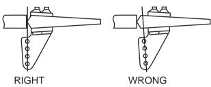
3. Repeat step # 1 - # 2 to install the control horn on the opposite aileron.
