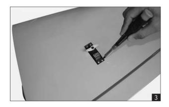
5. Repeat step # 2 - # 4 to install the second aileron servo in the opposite wing half.
