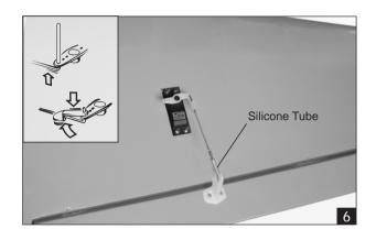
Repeat step # 4 - # 8 to install the second aileron linkage. After both linkages are completed, connect both of the aileron servo leads using a Y-harness you have purchased separately.
