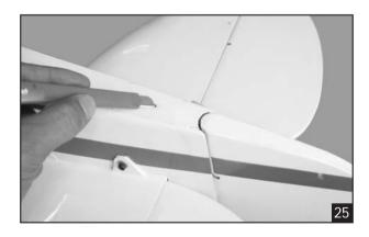
3. Secure the plate to the rudder.
