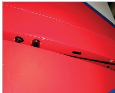
With a slightly firmer pressure in the direction of the fuselage, the „Clip Fixing“ wing securing device snaps into place immediately. This can be released later with a wedge for disassembly or by applying gentle pressure against the wing when holding the fuselage in place.
