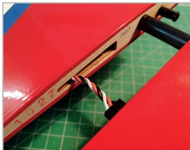
Finally, connect your receiver to the servos and controller according to the connection diagram of the transmitter manufacturer. The receiver can be fixed at the rear end, underneath the canopy frame, with e.g. Velcro tape.
