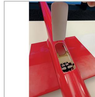
The fuselage floor lid can then be fastened with UHU Por. Make sure that all servo connectors and the receiver-side controller cable are facing forward towards the battery compartment so that they can be connected to the receiver later.
