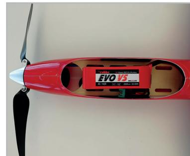
The recommended 4S 2600mAh battery finds its central place on the battery board and can be moved over a wide range for center of gravity adjustment. The mounting can be done according to individual preferences. We recommend Velcro tape and, in addition to securing, to insert Velcro cable ties through the slots of the battery board. This keeps the battery securely in position.
