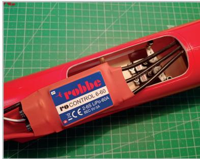
The controller is pushed under the battery board via the fuselage bottom access and connected to the motor.
