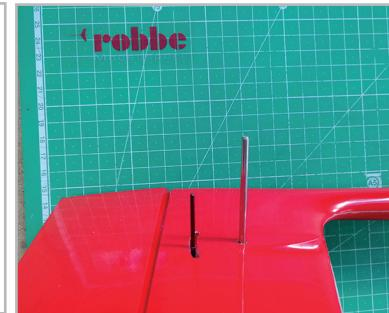
The two halves are attached to the fuselage by two steel wires. It is sufficient to tap both ends of the thicker steel wire flat with a hammer. Only so much that the tail halves are no longer loose, but also not too difficult to attach.
