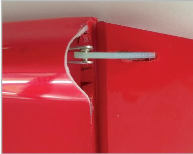
Afterwards the boom must first be guided through the boom connection on the servo side in order to be able to be hooked into the rudder.
