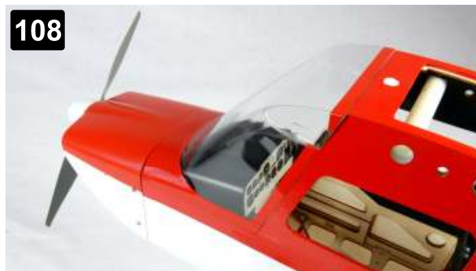
108 Kabinu osadíte na trup. No nevypadá báječně? Install the windshield on the fuselage. Does not it looks wonderful?
