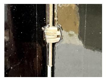
3. Press the top 90-degree bend of the rudder wire into the cutout on the top of the rudder.
