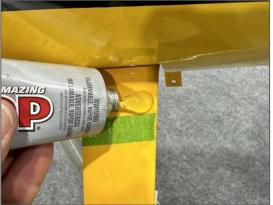
3. Slide the gear cuff back up into place. Tape over the bottom of cuff to ensure no residual adhesive runs down the landing gear. Also tape the top of the cuff to the fuselage to keep it in place while the adhesive sets.
