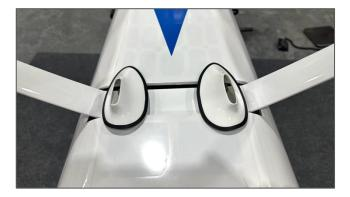
The landing gear cuffs are glued to the landing gear itself, and not the fuselage. This allows for easy removal of the landing gear.
