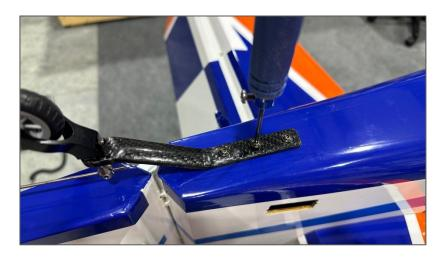
2. You can trim the steering wire leaving some overhang. Ensure that the steering wire stays on track within the ball link throughout the rudders full range of motion.
