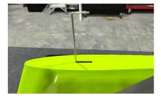
2. Run the wire through the top of the rudder through the hinges.
