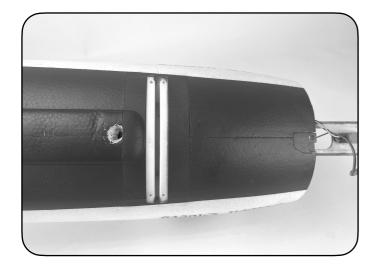
7. Using 1/4" or 6mm drill make a hole in the fuselage behind the front mounting plate as shown in the picture above. Alternately you can use a soldering iron or heat a piece of tubing to melt a hole through the foam. This hole will be used to run the LED and water rudder servo leads.
