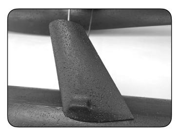
4. Glue the rear fairings onto the rear struts using 15 minute epoxy. Alternately you can leave these off for now and glue them on after you have assembled the floats to the fuselage.
