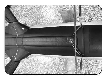
8. Mount the floats to the fuselage using the retaining plates and screws that you removed in step 6. Once you have the floats mounted run the wires into the fuselage through the hole you drilled in step 7. Note: Do not use tape to retain the wires anywhere that there is paint as the paint will come off the model when you remove the tape.
