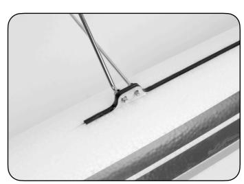
2. Slide the struts through the wood mounts in each of the floats. Note that the 5mm diameter bent struts go to the forward-most hole in the front of the float and the rear-most hole in the rear of the float, and they both angle towards the center (narrower gap) as they near the fuselage. The 4mm straight spreaders should go in the holes nearest the middle of the floats.
