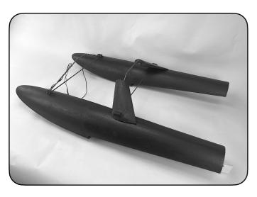
Secure the LED power wires and the water rudder servo lead to the front struts using clear tape or small tie straps. Once this is complete the floats should look like the picture above and are ready to install on the fuselage.
