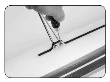
3. Secure the set screws to the struts on the outside of the plywood mounts. Pay special attention to the size of the strut and inside diameter of the wheel collars.
