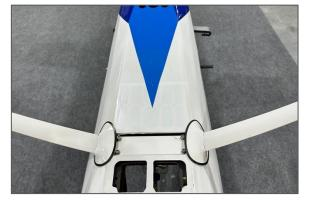
4. Keep airframe upright and allow the adhesive to cure for 24 hours (if using GOOP).
