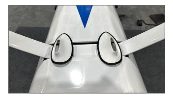
The landing gear cuffs are glued to the landing gear itself, and not the fuselage. This allows for easy removal of the landing gear.
