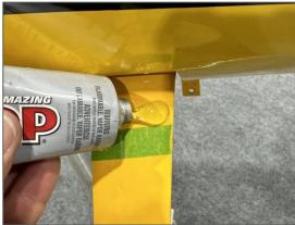
3. Slide the gear cuff back up into place. Tape over the bottom of cuff to ensure no residual adhesive runs down the landing gear. Also tape the top of the cuff to the fuselage to keep it in place while the adhesive sets.
