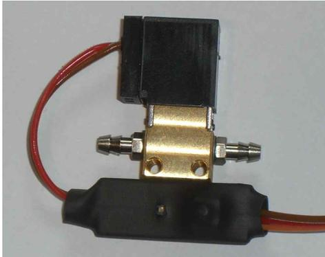
This valve is attached directly to the receiver to control smoke liquids.
