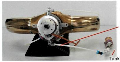
Connect the tube from the fuel pump to the lower connector in front of the gearbox. Consider in case the engine is mounted upside down the connectors even are changed.
