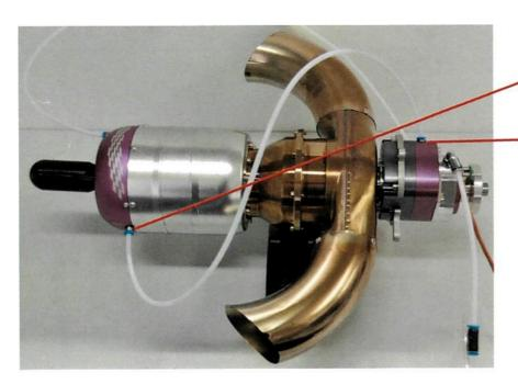
Make sure the connector "Lube to Gearbox" is connected to the gearbox as shown on the picture
