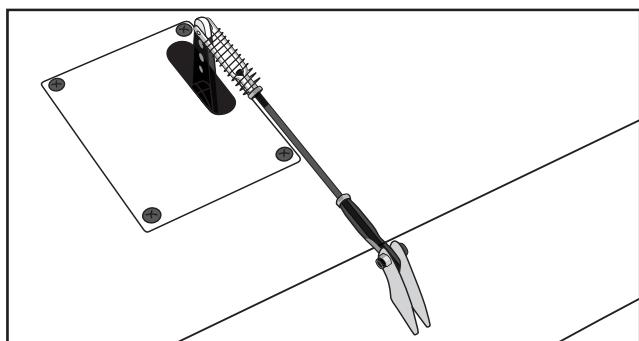
After both linkages are completed, connect both of the aileron servo leads using a Y-harness you have purchased.
