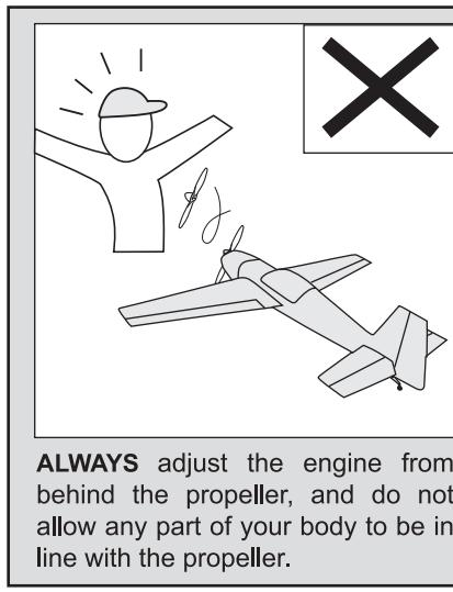
**ALWAYS** adjust the engine from behind the propeller, and do not allow any part of your body to be in line with the propeller.
