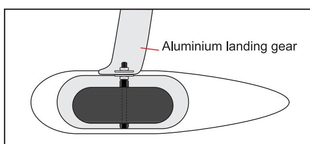
1) Assemble and mounting the wheel pants as shown in the following pictures.
