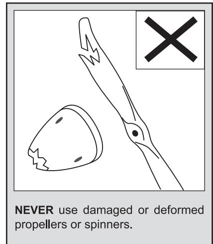
**NEVER** use damaged or deformed propellers or spinners.
