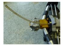
Figure no. 7 – Tube is used for crankcase ventilation and as a drain of superfluous oil. **Tube must remain free. Do not reduce its cross section or extend!**
