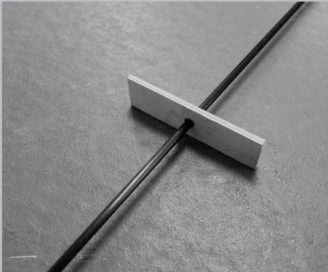
The plywood guide for the linkage is glued with epoxy to about half the length of the linkage between the fuselage sidewalls.
