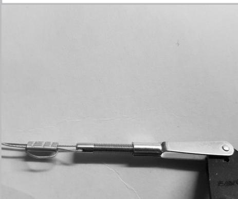
First thread a ferrule onto the rope and pass it through the hole of an eyebolt and back through the ferrule. Pay attention to a short length of eyelets. Both sides can now be pressed on the rudder horn of the rudder by pliers.
