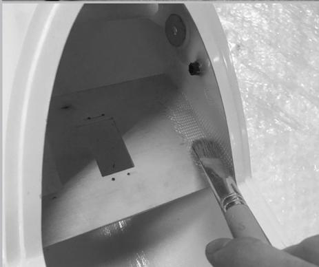
Now the servo board can also be glued into the previously determined location in the fuselage. To do this, the elevator linkage should be suspended with a neutral rudder and 90 ° servo lever. The fuselage side walls must be sanded accordingly before. We recommend to reinforce the gluing by a layer of 160g fabric.
