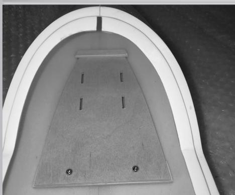
The receiver and the batteries should be placed as far forward in the fuselage as possible and well secured. Therefore, glue in the wooden battery tray supports and fix the battery tray by screws. The batteries can be fixed by velcro and velcro loops.
