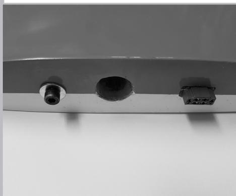
For the electrical connection fuselage / wing we recommend the 6-pin Multiplex connectors, which can be either loose or permanently installed. The fixed installation requires a bit more effort at the beginning, but facilitates the assembly of the SWIFT later on the airfield enormously.
