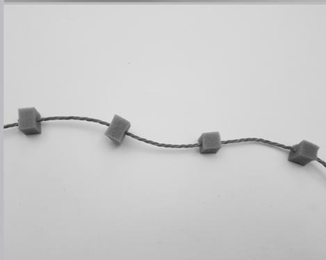
To avoid subsequent rattling of the servo cables in the wing, it is advisable to provide the cable with foam pieces.
