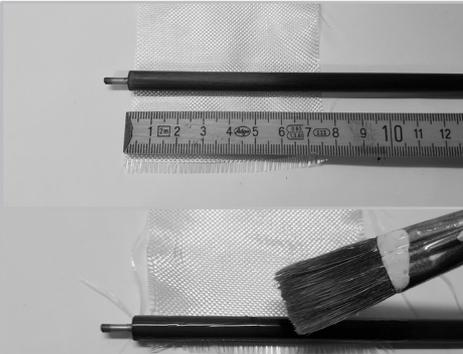
Optional: In order to avoid bursting of the tube under high loads, the tube should be reinforced on both sides with glass fabric. For this purpose, after sanding both ends are wrapped twice with soaked 80g glass mat.
