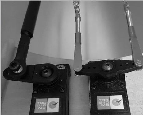
Screw the elevator and rudder servo into the slots provided in the servo board. The servo lever of the elevator should be approx. 18mm long until the bore, the rudder lever needs approx. 45mm length (bore / bore). Both servo levers should be aligned at 90 ° neutral position.
