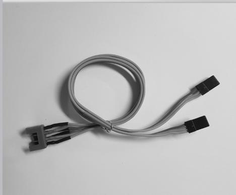
Solder the approx. 50cm long servo cable to the contacts of the MPX connectors.
