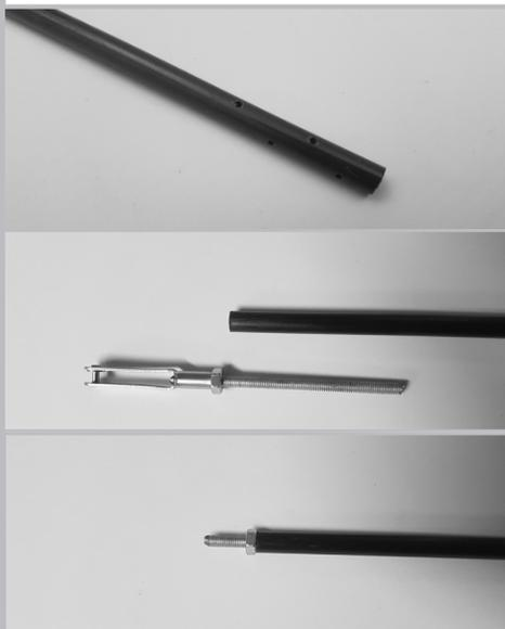
Make the elevator linkage from the carbon tube, M3 threaded rods, M3 nuts and M3 clevises in the previously determined length. Equip the carbon push rod with 2-3 cross holes with a 1.5 mm drill bit. This achieves a positive-locking connection by the glue. Bonding the threads to the carbon tube should be done with Uhu Endfest 300 or thickened 24h epoxy resin after the threads have been properly degreased. The threads must be about 25mm out of the pipe. Do not use inferior adhesives!
