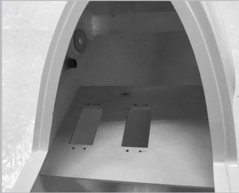
Start by adjusting the servo board in the fuselage. It should be glued in as far back as possible in front of the wing joiner tube. Do not glue now!
