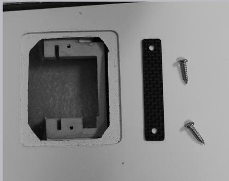
Begin by installing the aileron and flap servos in the brackets. Attach the servos with the carbon tabs and wood screws. Pull the servo cables into the wing and solder them to the servos.
